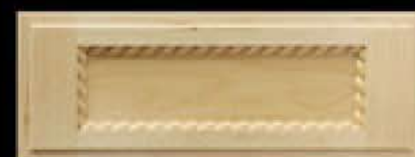
DFFP RQ \frac{5}{16} " in Soft Maple Minimum Width 6\frac{1}{2} " Minimum Height 4\frac{3}{4} " Stiles 2\frac{3}{8} " • Rails 1\frac{3}{8} " DF Thickness \frac{13}{16} "
