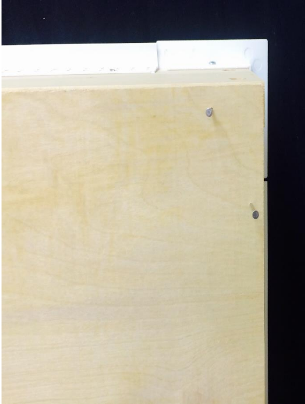
Image 1 nailing on the back panel
